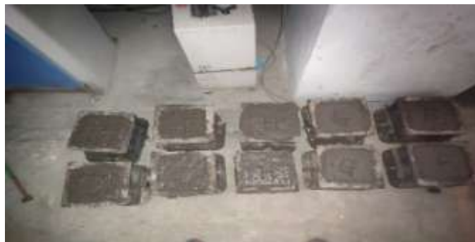
Figure No. 2(Cube Casting)
